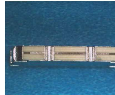
Sn/Pb Plated and Fusion Processed Hybrid Coupler
