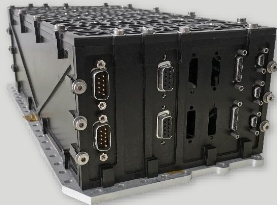
PT2020 / INFANTE Power sub-system
