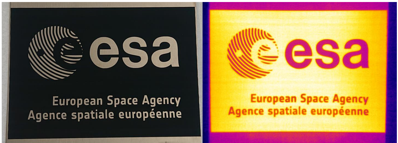
BLAST treated aluminum (visible spectrum – left; infrared - right)
